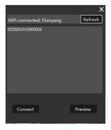
The thermal imaging camera WiFi will show here, select the thermal imaging camera to be connected, and then click the connect button. If a password dialog box pops up, check the
