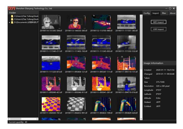
At this time, the pictures in the software image preview area are still in the thermal imaging camera. Select the images, right-click and download, and you can download the thermal imaging to the "Picture" directory of the software installation directory.
