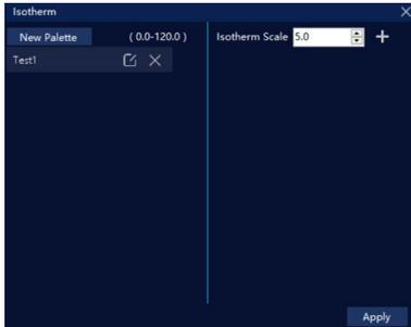
(3) The isotherm color blocks can be added on the right side. Different isotherm color blocks can be added by clicking "+" following the width of the temperature line.
