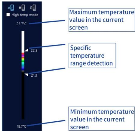
Specific temperature range detection: Users can adjust the temperature range screens that they desire to focus on according to their own needs. The data can be adjusted with the up and down arrows. When the temperature is above the observed maximum temperature, it is displayed in white, and when the temperature is below the minimum temperature, it is displayed in black. The screen of Specific temperature range detection is assigned with colors according to the color palette.
