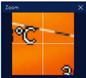
Window amplifying function: small objects can be amplified for 6 times with the mouse.
