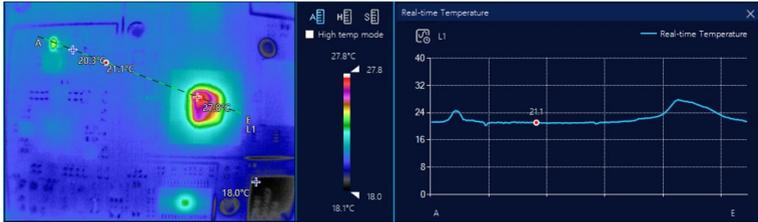
Click on any point on the right line to mark the corresponding point and temperature in the left video. As shown below:
