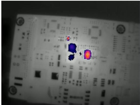
Extended dynamic temperature bars are often used in detection of leakage and short-circuit of the circuit boards.
