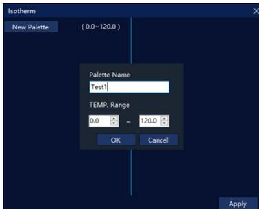
(2) Enter the palette name of the isotherm color board and the fixed temperature range of the isotherm color board. Press "OK" and store it as an isotherm template. It will work for the thermal analysis video after the application.
