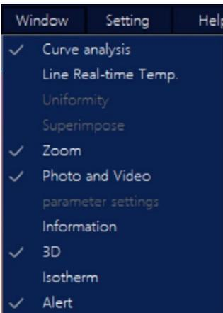
Window function, which can display different function windows on the interface. The thermal analysis video window always exists, and other function windows can be closed and opened.
