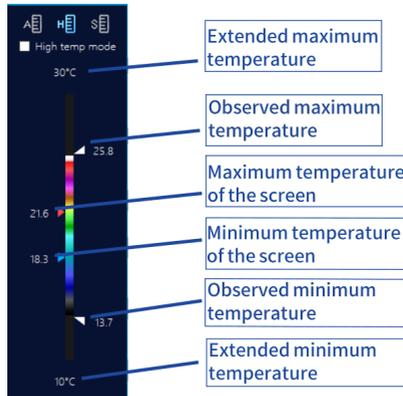
The users can pull the arrows of observing the maximum temperature and the minimum temperature, and focus on the images of the temperature range of concern. The images outside the observing temperature segment are in black and white. As shown below:
