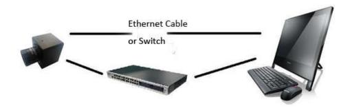
To connect infrared thermal camera with PC through Ethernet cable or switch, the IP address is "192.168.1.x", x is not the same as the camera, and the subnet is "255.255.255.0" Open the analysis software, to scan the camera in the left side, then connect the camera,
