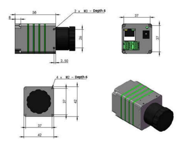
Figure: SR series dimension (mm)
