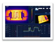
Analysis of temperature change process of heating materials under different voltages and currents
