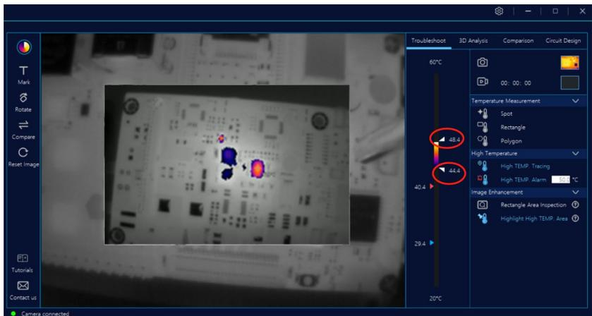
As shown below, there are 4 suspected leakage points.
